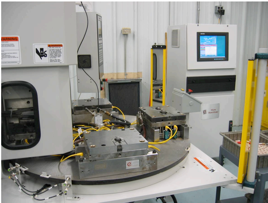
Figure 2. Process Control System to adjust for 50% variation in encapsulant volume
